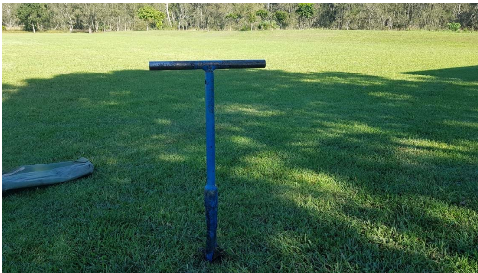
Plate 3.2 Soil samples were obtained using a hand auger, photo taken looking south from PDHP building 1
