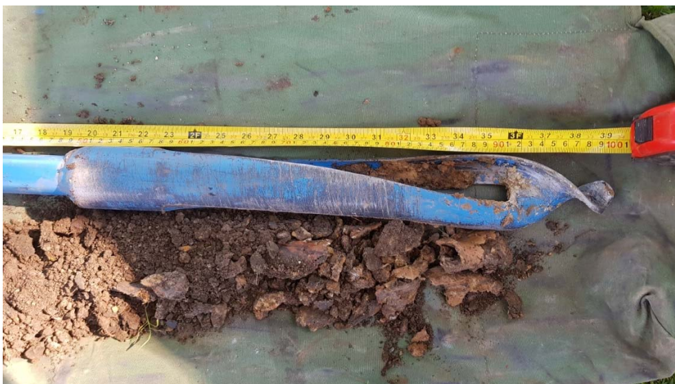
Plate 3.3 Example of soil profile consisting of granular to light clay fill, photo taken from BH4 (PDHP building 2).
